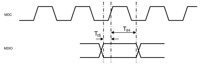
Figure 23. Reception Data Timing of SMI Interface
