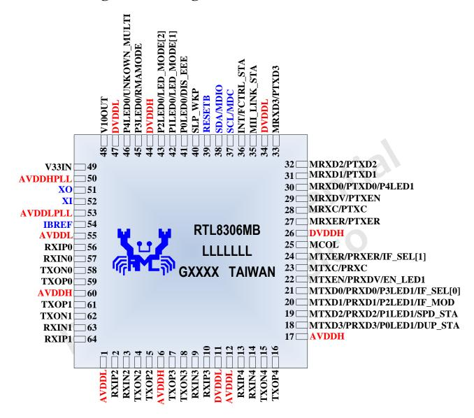
Figure 2. Pin Assignments
