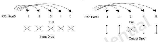
Figure 20. Broadcast Input Drop vs. Output Drop
