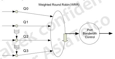
Figure 17. Packet-Scheduling Diagram
