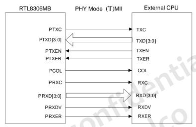
Figure 10. PHY Mode (T)MII Signal Diagram
