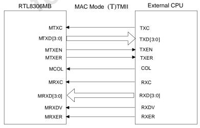
Figure 11. MAC Mode (T)MII Signal Diagram
