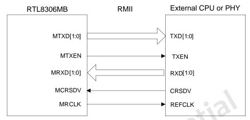
Figure 12. RMII Signal Diagram
