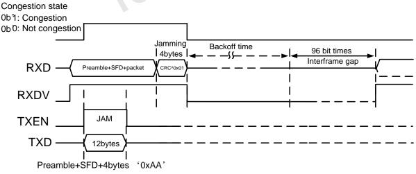
Figure 3. Collision-Based Back Pressure Signal Timing
