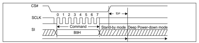
Figure21a. Deep Power-Down Sequence Diagram (QPI)
