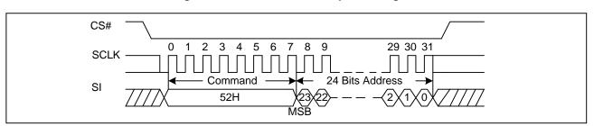
Figure18a. 32KB Block Erase Sequence Diagram (QPI) CS# 0 SCLK Command 52H A12-8 A23-16 12  $IO_0$ 9 5  $IO_1$ 6 IO<sub>2</sub> IO<sub>3</sub>
