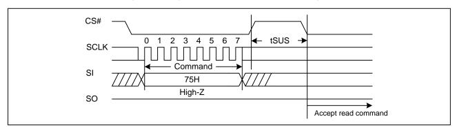
Figure 28. Program/Erase Suspend Sequence Diagram
