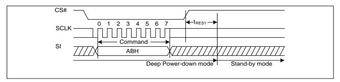
Figure22a. Release Power-Down Sequence Diagram (QPI)
