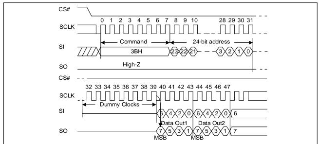
Figure9. Dual Output Fast Read Sequence Diagram
