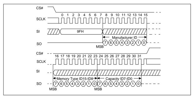
Figure27. Read Identification ID Sequence Diagram
