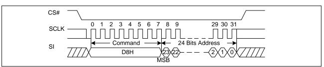
Figure19. 64KB Block Erase Sequence Diagram
