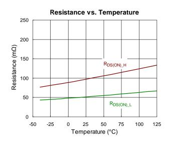
Figure 13. RT6253A/B RDS(ON) vs. Temperature
