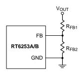
Figure 2. Output Voltage Setting
