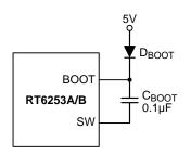
Figure 10. External Bootstrap Diode
