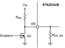
Figure 8. Digital Enable Control Circuit
