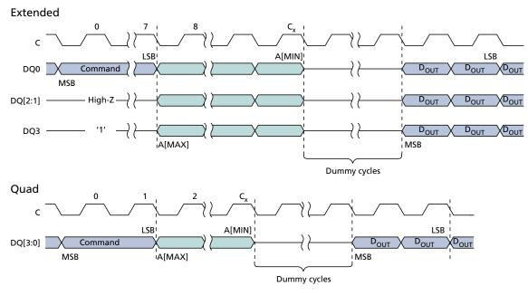
otes: 1. For extended protocol,  $C_x = 7 + (A[MAX] + 1)/4$ ; For quad protocol,  $C_x = 1 + (A[MAX] + 1)/4$ .
