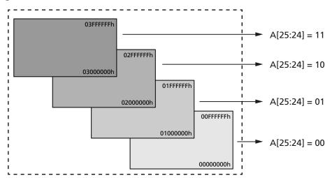
The PROGRAM and ERASE operations act upon the 128Mb segment selected in the extended address register. The BULK ERASE operation erases the entire device.
