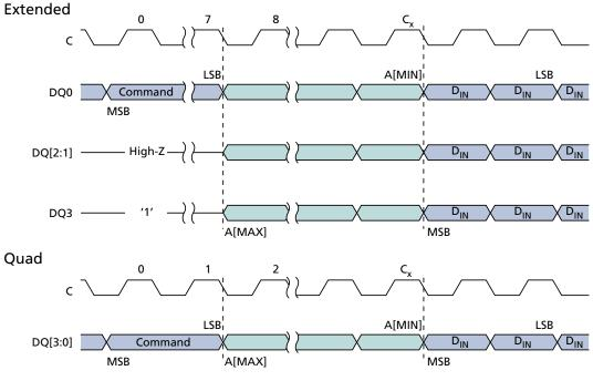
Notes: 1. For extended SPI protocol,  $C_x = 7 + (A[MAX] + 1)/4$ ; For quad SPI protocol,  $C_x = 1 + (A[MAX] + 1)/4$ .
