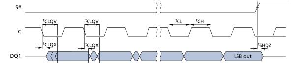
**Figure 56: Output Timing for DTR**
