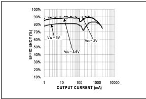
FIGURE 2-1: Efficiency vs. Output Current ( $V_{OUT} = 1.8V @ 25^{\circ}C$ ).
