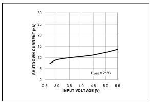
FIGURE 2-5: Shutdown Current vs Input Voltage.
