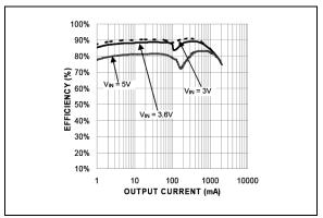
**FIGURE 5-2:** Efficiency Under Load  $V_{OUT} = 1.8V @ 25^{\circ}C$ .
