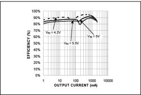
FIGURE 2-2: Efficiency vs. Output Current ( $V_{OUT} = 3.3V @ 25^{\circ}C$ ).
