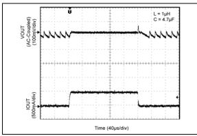
FIGURE 2-25: Load Transient (10 mA to 500 mA).
