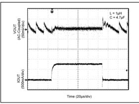
FIGURE 2-26: Load Transient (10 mA to 750 mA).
