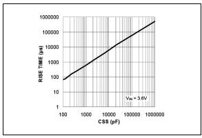
FIGURE 2-3: V<sub>OUT</sub> Rise Time vs. C<sub>SS</sub>.
