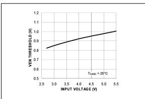
FIGURE 2-14: Enable Threshold vs. Input Voltage.
