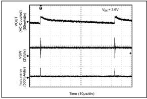
FIGURE 2-18: Switching Waveform Discontinuous Mode (Load = 1 mA).
