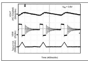
**FIGURE 2-20:** Switching Waveform Discontinuous Mode (Load = 50 mA).
