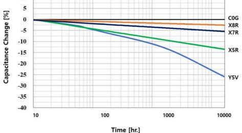
The capacitance value can be restored (a.k.a. 'de-aged') by exposing the component to elevated temperatures approaching its Curie Temperature (approximately 120°C). This 'deaging' can occur during the component's solder-assembly onto the PCB, during life or temperature cycle testing., or by ' baking ' at 150°C for about 1 hour.
