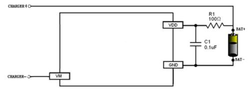
Fig 6 XB3153IS in a Typical Battery Protection Circuit
