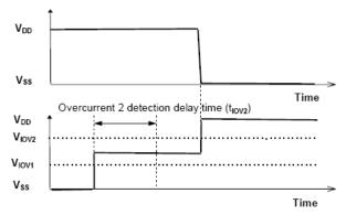
Figure 4. Overcurrent delay time
