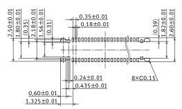
Recommended metal mask pattern Metal mask thickness: When 100 μm (Signal terminal opening ratio: 70%) (Power terminal opening ratio: 77%)
