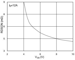
Fig.2 On-Resistance vs. G-S Voltage
