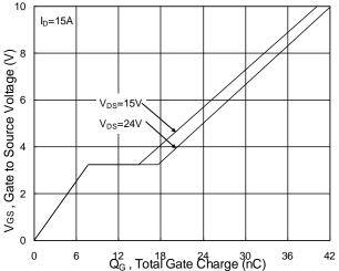
Fig.4 Gate-Charge Characteristics
