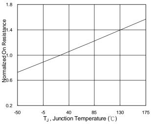
Fig.6 Normalized  $R_{\text{DSON}}$  vs.  $T_{\text{J}}$
