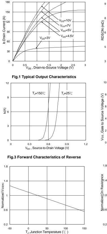
Fig.5 Normalized V<sub>GS(th)</sub> vs. T<sub>J</sub>
