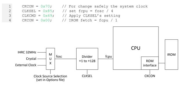
ROM interface is built in between CPU and IROM (program memory). It optionally extends the data fetching cycle in order to support lower speed program memory.
