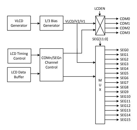
In LCD mode, the LCD builds in one internal bias circuit to adjust LCD power and bias voltage. There are 16-pin GPIO shared with COM pins and SEG pins which controlled by LCDSEG and LCDSEG1 registers. The LCD builds in POCON/P1CON/P2CON/P3CON registers to set pure analog input pin. After setup LCDEN bit, the LCD starts output analog data. In static mode, the selected COM/SEG pins switch to like GPIO output mode and only output OV and VDD voltage.
