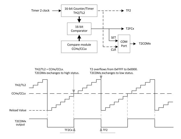
By contrast, the indirectly output method is an event which keep the mapped pin's previous output setting until Timer 2 counter overtakes CRC/CC1/CC2/CC3 register value. In this mode, the transition of the output signal can be configured by software. In other word, the P0.0 register bit would be affect T2COM0/P0.0 pin when TH2/TL2 equal to CRC registers. A Timer 2 overflow causes no output change.
