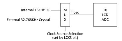
In external 32.768 kHz crystal mode, LXIN and LXOUT pin switch to crystal mode to drive an off-chip 32.768 kHz crystal after LCKS bit is cleared. Microcontroller supplies WARM bit (the 4<sup>th</sup> bit of PFLAG) to indicate crystal warm-up status. The WARM bit is set when crystal warm-up procedure ready and cleared when crystal stop. If 32.768 kHz crystal is abnormal stop, re-clear LCKS bit can re-start crystal warm-up procedure.
