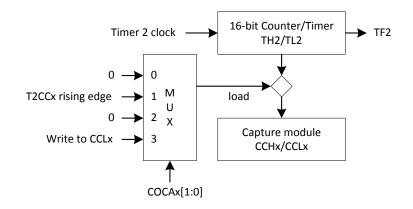
The split event can from hardware or software. The T2CCO pin (shared with P0.5) can trigger a hardware split event that duplicates TH2/TL2 value to CRCH/CRCL registers, whereas T2CC1 (P0.6), T2CC2 (P0.2) and T2CC3 (P0.3) respectively control CC1 to CC3 registers.
