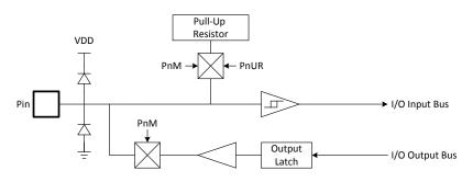
Bi-direction I/O Pin Shared with Specific Digital Input Function, e.g. INT2.
