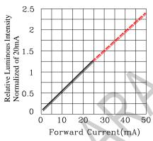
Fig.4 Relative Luminous Intensity vs.Forward Current
