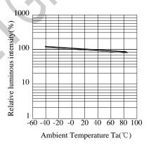
Fig.5 Luminous Intensity vs. Ambient Temperature
