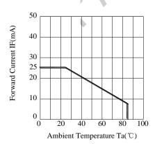
Fig.6 Forward Current Derating Curve
