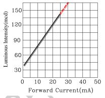
Fig.3 Luminous Intensity vs.Forward Current
