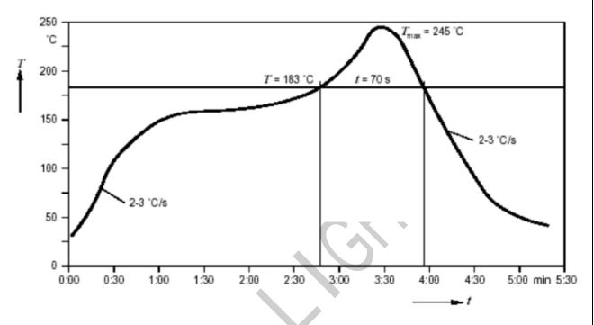
• Suggest Pb-Free IR Reflow Soldering Profile Condition:
