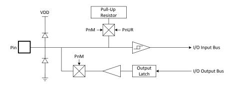
Bi-direction I/O Pin Shared with Specific Digital Input Function, e.g. INTO, UART.
