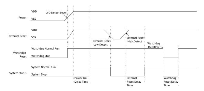
The power stabilization period spends 4.6 ms in typical condition. Afterward the microcontroller fetches CPU Clock Source selection automatically. The selected clock source would be driven, and the system counts 2048 times of the clock period and 5 times of the internal low-speed oscillator clocks to ensure its reliability.
