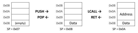
By default, stack pointer (SP register) points to 0x07 which means the stack area begin at IRAM address 0x08. In other word, if a planned stack area is assigned from IRAM address 0xC0, the appropriate SP register is anticipated to set at 0xBF after system reset.
