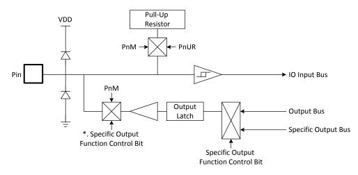
$\scriptstyle *.$  Some specific functions switch I/O direction directly, not through PnM register.
