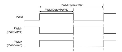
The PWM has frequency mode to change PWM output frequency. The frequency mode is controlled by PWO[5:0]. When PWOn=1, PWMn pin outputs 1/2\*frequency PWM signal. When PWOn=0, PWMn pin outputs 1\*frequency PWM signal.
