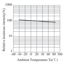
Fig.5 Luminous Intensity vs. Ambient Temperature
