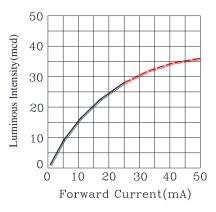
Fig.3 Luminous Intensity vs.Forward Current
