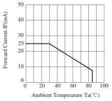
Fig.6 Forward Current Derating Curve
