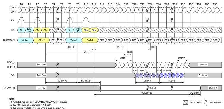
3. The minimum number of clock cycles from the burst write command to the burst write command for any bank is BL/2
