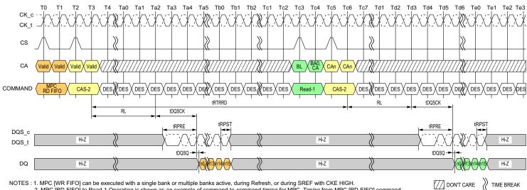
2. MPC [RD-FIFO] to Read-1 Operation is shown as an example of command-to-command timing for MPC. Timing from MPC [RD-FIFO] command
