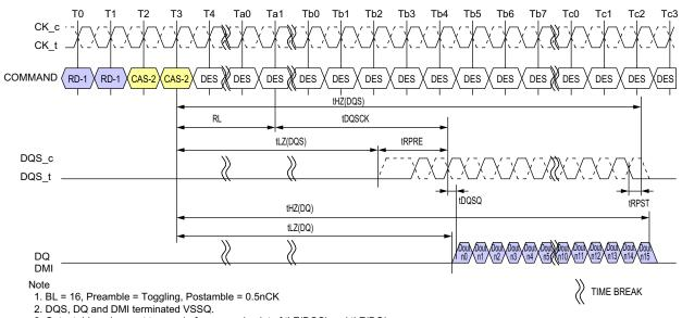
3. Output driver does not turn on before an end point of tLZ(DQS) and tLZ(DQ).
