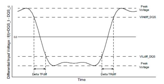
NOTES : 1. Differential signal rising edge from VILdiff\_DQS to VIHdiff\_DQS must be monotonic slope. 2. Differential signal falling edge from VILdiff\_DQS to VIHdiff\_DQS must be monotonic slope.
