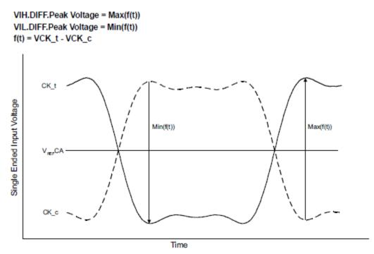
Note : 1.  $V_{REF}CA$  is LPDDR4 SDRAM internal setting value by  $V_{REF}$  Training.
