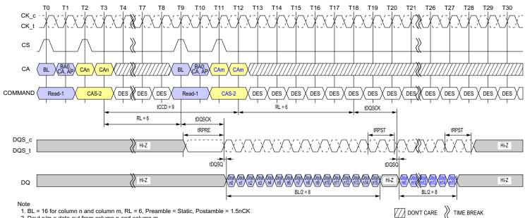
2. Dout n/m = data-out from column n and column m.
