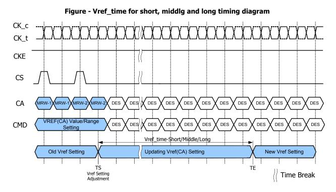
The MRW command to the mode register bits are as follows.
