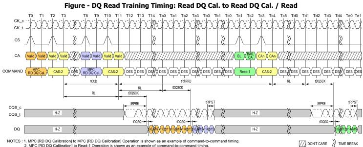
2. MPC [RD DQ Calibration] to Read-1 Operation is shown as an example of command-to-command timing.
