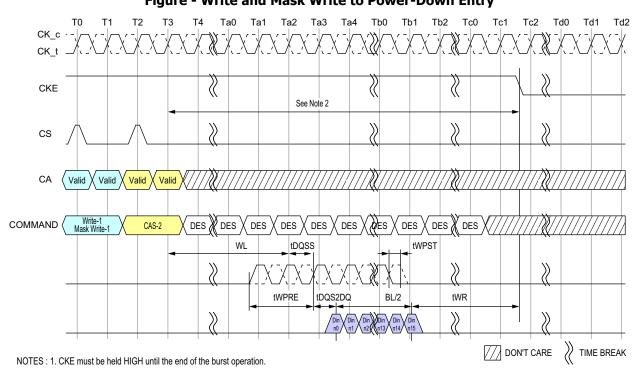
Figure - Write and Mask Write to Power-Down Entry
