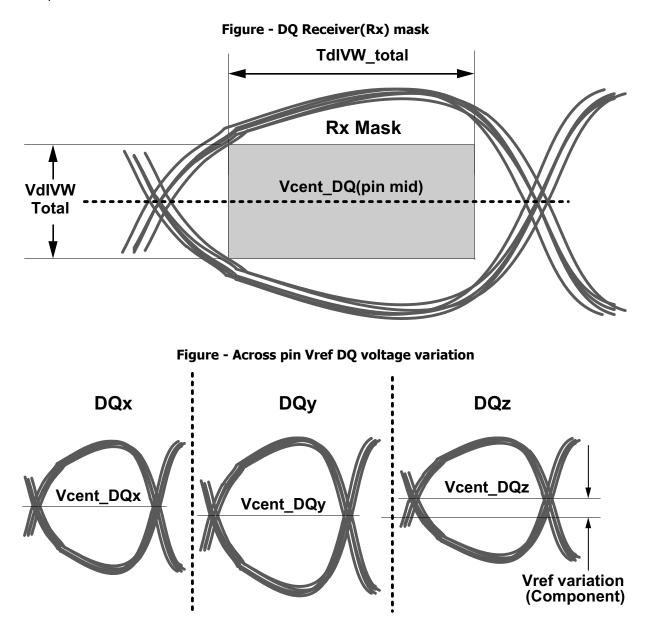
Vcent\_DQ(pin\_mid) is defined as the midpoint between the largest Vcent\_DQ voltage level and the smallest Vcent\_DQ voltage level across all DQ pins for a given DRAM component. Each DQ Vcent is defined by the center, i.e. widest opening, of the cumulative data input eye as depicted in the above figure. This clarifies that any DRAM component level variation must be accounted for within the DRAM Rx mask. The component level VREF will be set by the system to account for Ron and ODT settings.
