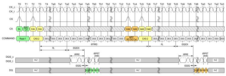
NOTES : 1. Read-1 to MPC [RD DQ Calibration] Operation is shown as an example of command-to-command timing.
