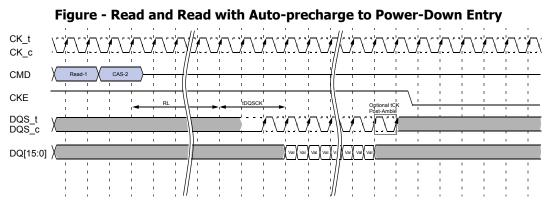
1. CKE must be held HIGH until the end of the burst operation.
