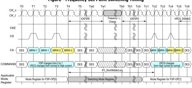
Figure - Frequency Set Point Switching Timing
