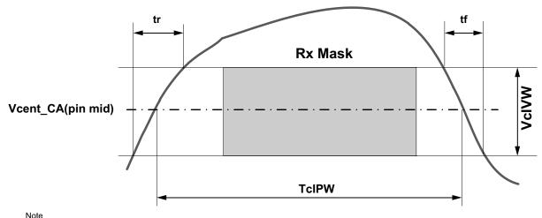
Figure - CA TclPW and SRIN\_clVW definition (for each input pulse)
