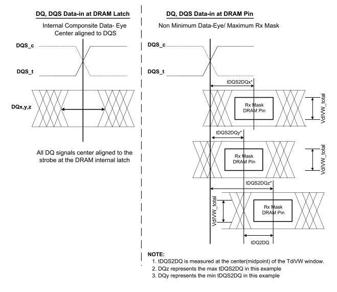
All of the timing terms in DQ to DQS t are measured from the DQS\_t/DQS\_c to the center(midpoint) of the TdIVW window taken at the VdIVW\_total voltage levels centered around Vcent\_DQ(pin\_mid). In the above figure the timings at the pins are referenced with respect to all DQ signals center aligned to the DRAM internal latch. The data to data offset is defined as the difference between the min and max tDQS2DQ for a given component.
