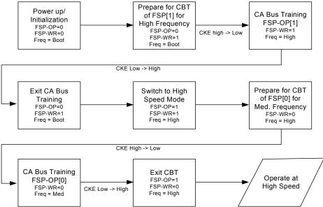
Once both Frequency Set Points have been trained, switching between points can be performed by a single MRW followed by waiting for tFC (figure below)
