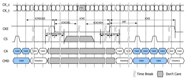
1. Input clock frequency can be changed or the input clock can be stopped or floated during power-down, provided that upon exiting power-down, the clock is stable and within specified limits for a minimum of RU(tCKCKEH/tCK) of stable clock prior to power-down exit and the clock frequency is between the minimum and maximum specified frequency for the speed grade in use.
