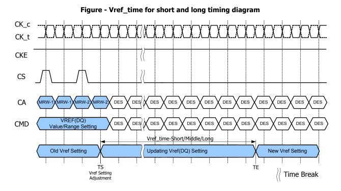
The MRW command to the mode register bits are as follows.
