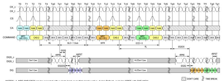
NOTES : 1. MPC [WR FIFO] can be executed with a single bank or multiple banks active, during Refresh, or during SREF with CKE HIGH. 2. MPC [WR-FIFO] to MPC [RD-FIFO] is shown as an example of command-to-command timing for MPC. Timing from MPC [WR-FIFO] to MPC [RD-FIFO] is specified in the command-to-command timing table.
