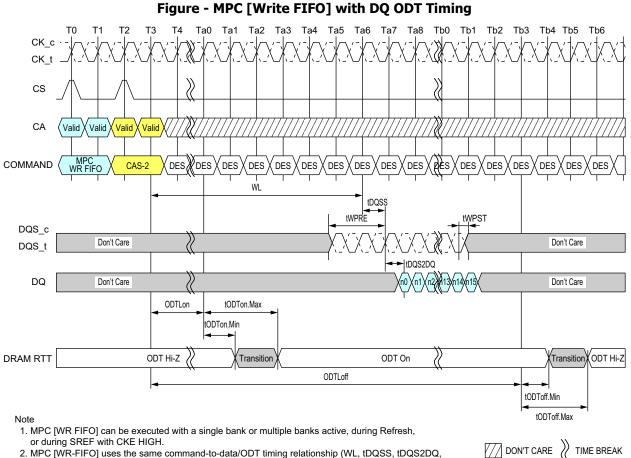
2. MPC [WR-FIFO] uses the same command-to-data/ODT timing relationship (WL, tDQSS, tDQS2DQ, ODTLon, ODTLoff, tODTon, tODToff) as a Write-1 command.
