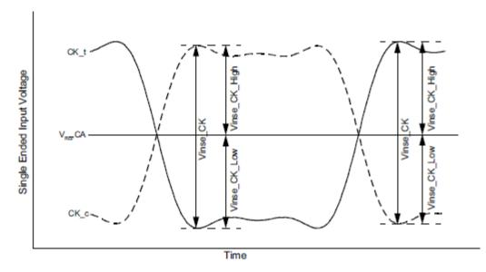
Figure - Clock Single-Ended Input Voltage
