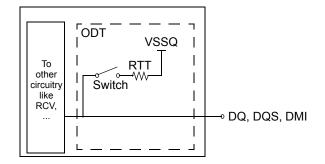
Figure - Functional Representation of DQ ODT
