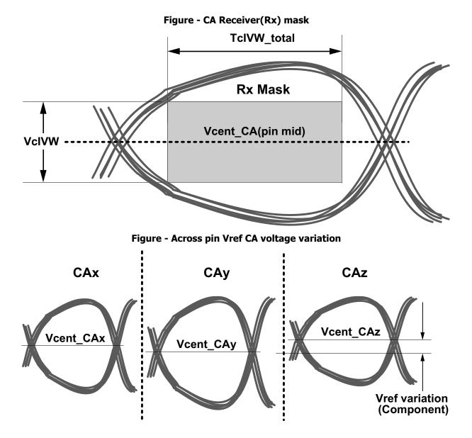
Vcent\_CA(pin avg) is defined as the midpoint between the largest Vcent\_CA voltage level and the smallest Vcent\_CA voltage level across all CA and CS pins for a given DRAM component. Each CA pin Vcent level is defined by the center, i.e. widest opening, of the cumulative data input eye as depicted in the above figure. This clarifies that any DRAM component level variation must be accounted for within the DRAM CA Rx mask. The component level Vref will be set by the
