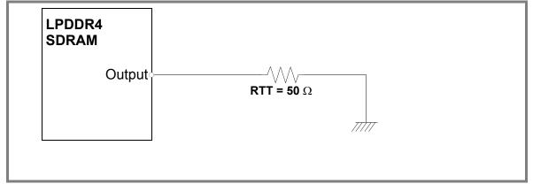
Note: 1. All output timing parameter values (like  $t_{DQSCK}$ ,  $t_{DQSQ}$ ,  $t_{QHS}$ ,  $t_{HZ}$ ,  $t_{RPRE}$  etc.) are reported with respect to this reference load. This reference load is also used to report slew rate.
