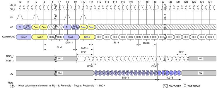
Dout n/m = data-out from column n and column m.
