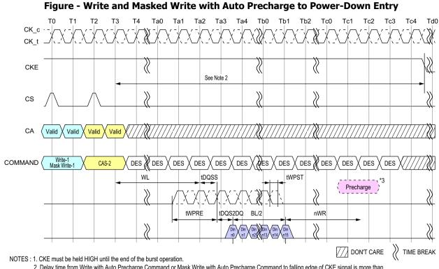
Delay time from Write with Auto Precharge Command or Mask Write with Auto Precharge Command to falling edge of CKE signal is more than (WL x tCK) + tDQSS(Max) + tDQS2DQ(Max) + ((BL/2) x tCK) + (nWR x tCK) + (2 x tCK)
