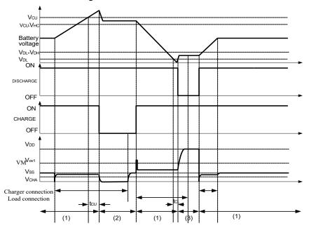
Figure 5-1 Overcharge and Overdischarge Voltage Detection
