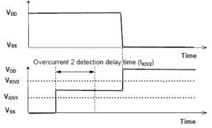
Figure 4. Overcurrent delay time
