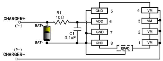
Fig 6 XB8886G in a Typical Battery Protection Circuit
