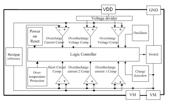
Figure 3. Functional Block Diagram
