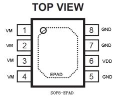
Figure 2. PIN Configuration
