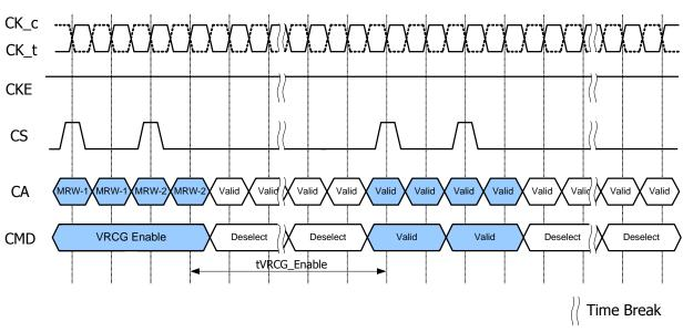
Figure - VRCG Enable timing
