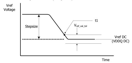
Figure - Vref full step from Vrefmin to Vrefmax case
