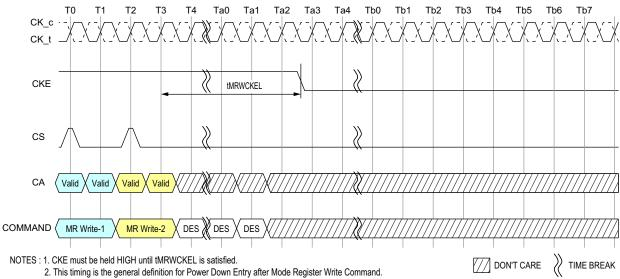
2. This timing is the general definition for Power Down Entry after Mode Register Write Command. When a Mode Register Write Command changes a parameter or starts an operation that requires special timing longer than tMRWCKEL, that timing must be satisfied before CKE is driven low.
