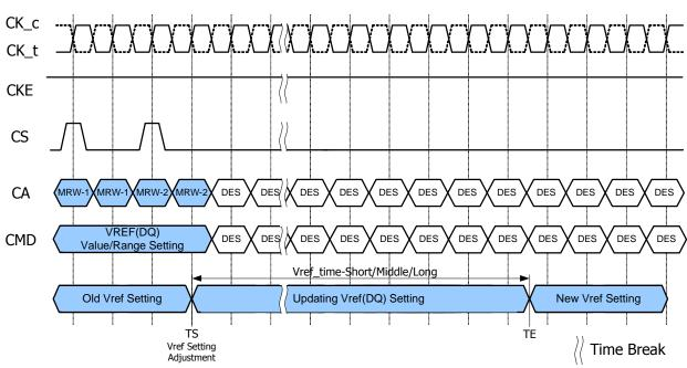
Figure - Vref\_time for short and long timing diagram
