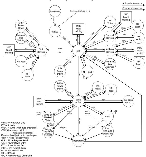
Figure - Simplified State Diagram
