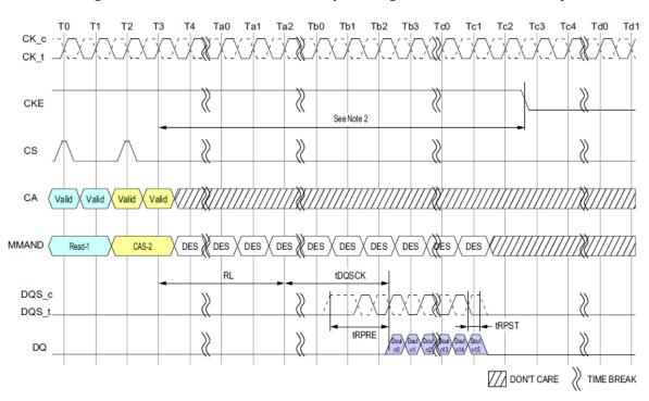
Figure - Read and Read with Auto-precharge to Power-Down Entry
