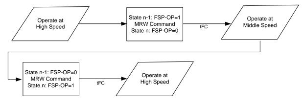
Switching to a third (or more) Set-Point can be accomplished if the memory controller has stored the previously-trained values (in particular the Vref-CA calibration value) and re-writes these to the alternate Set-Point before switching FSP-OP (Figure below).
