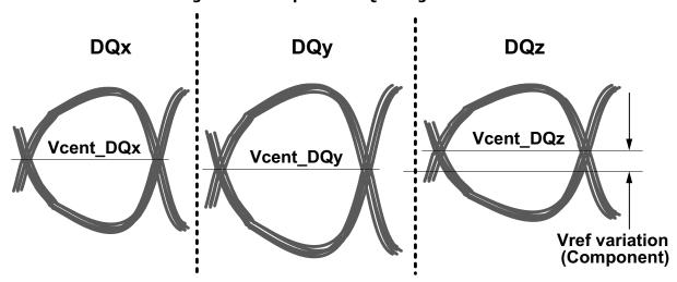
Vcent\_DQ(pin\_mid) is defined as the midpoint between the largest Vcent\_DQ voltage level and the smallest Vcent\_DQ voltage level across all DQ pins for a given DRAM component. Each DQ Vcent is defined by the center, i.e. widest opening, of the cumulative data input eye as depicted in the above figure. This clarifies that any DRAM component level variation must be accounted for within the DRAM Rx mask. The component level VREF will be set by the system to account for Ron and ODT settings.
