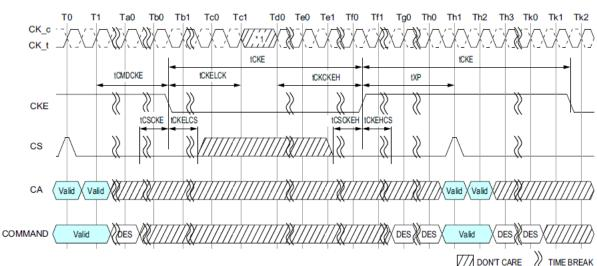
Figure - Basic Power-down Entry and Exit Timing
