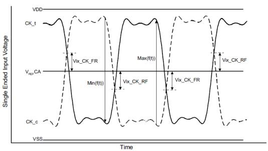
NOTES: 1. The base level of Vix\_CK\_FR/RF is V<sub>REF</sub>CA that is LPDDR4 SDRAM internal setting value by V<sub>REF</sub> Training.
