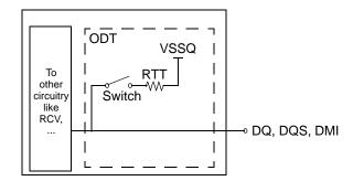
Figure - Functional Representation of DQ ODT
