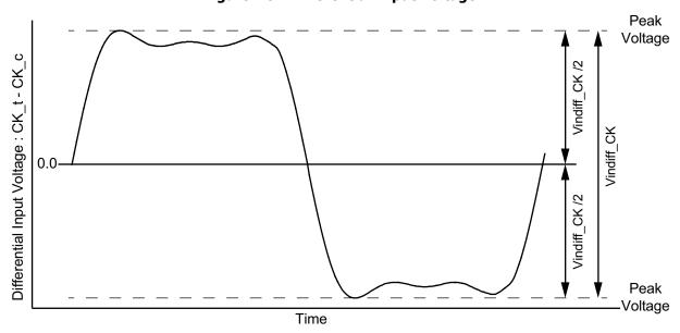
**Figure - CK Differential Input Voltage**
