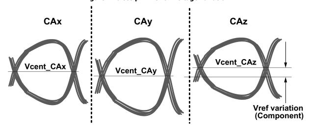
Vcent\_CA(pin avg) is defined as the midpoint between the largest Vcent\_CA voltage level and the smallest Vcent\_CA voltage level across all CA and CS pins for a given DRAM component. Each CA pin Vcent level is defined by the center, i.e. widest opening, of the cumulative data input eye as depicted in the above figure. This clarifies that any DRAM component level variation must be accounted for within the DRAM CA Rx mask. The component level Vref will be set by the
