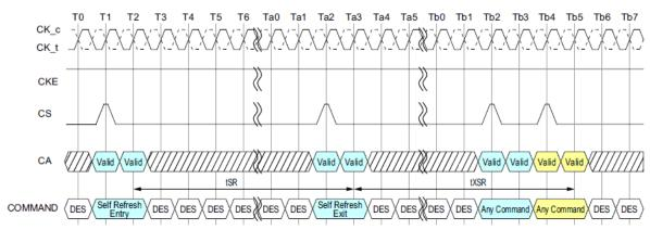
Figure - Self Refresh Entry/Exit Timing
