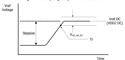
Figure - Vref step single stepsize increment case
