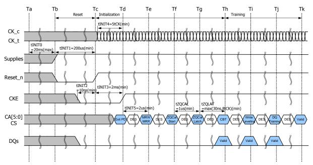
Figure - Power Ramp and Initialization Sequence
