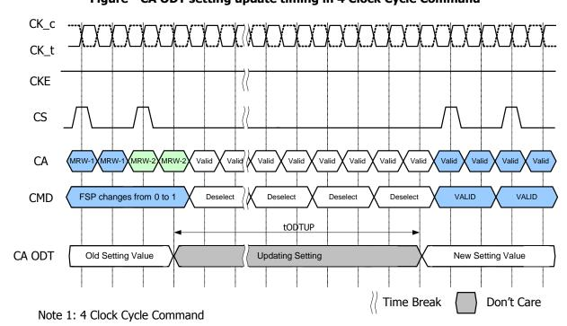
Figure - CA ODT setting update timing in 4 Clock Cycle Command
