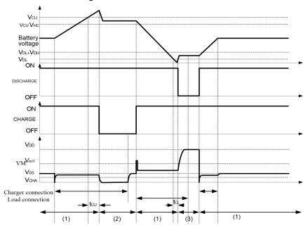
Figure 5-1 Overcharge and Overdischarge Voltage Detection
