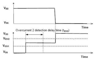
Figure 4. Overcurrent delay time
