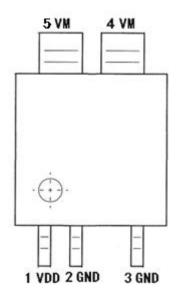
Figure 2. PIN Configuration(TOP View)
