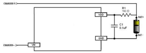
Fig 6 XB7608AJL in a Typical Battery Protection Circuit
