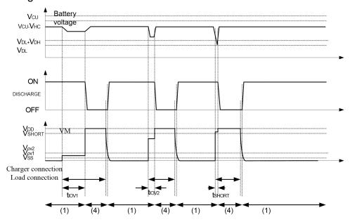
Figure 5-2 Overdischarge Current Detection
