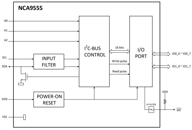
Fig 6. Block Diagram of NCA9555
