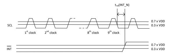
Fig 19. Parameter Measurement Waveform:  $t_{rst(INT\_N)}$
