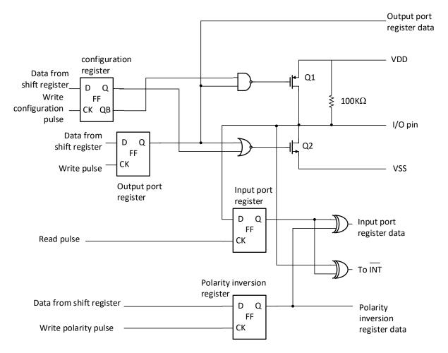
Fig 5. Simplified schematic of I/Os
