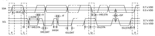
Fig 3. Definition of timing on I<sup>2</sup>C-bus
