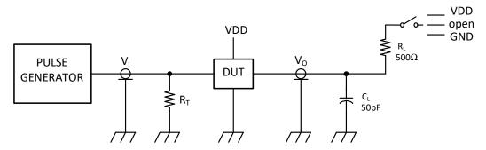
$R_L$  = load resistor.
