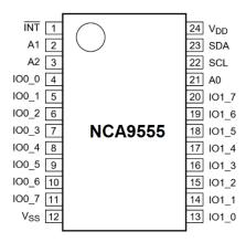
Figure 1. NCA9555 Block Diagram
