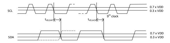
Fig 20. Parameter Measurement Waveform: tVD; DAT & tVD;ACK
