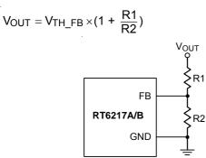
Figure 5. Output Voltage Setting
