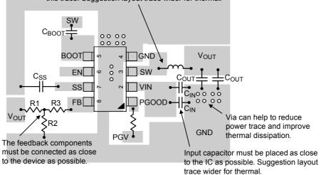
Figure 10. PCB Layout Guide
