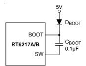
Figure 6. External Bootstrap Diode
