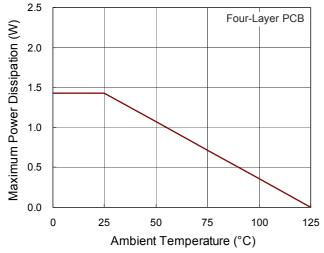
Figure 9. Derating Curve of Maximum Power Dissipation
