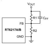
Figure 1. CFF Capacitor Setting
