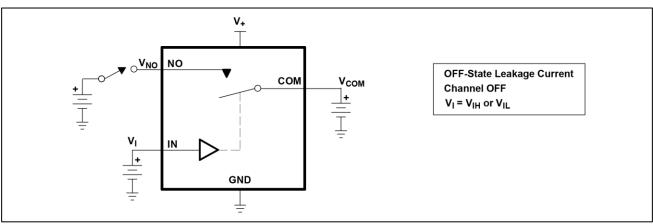
Figure 2.OFF-State Leakage Current (ICOM(OFF), INO(OFF))
