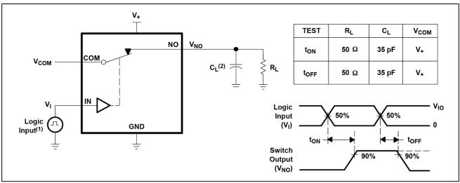
Figure 5.Turn-On (ton) and Turn-Off Time (toff)
