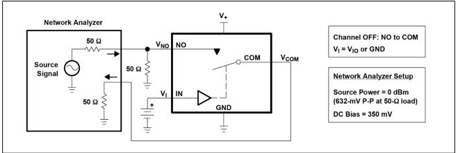
Figure 8.OFF Isolation (O<sub>ISO</sub>)
