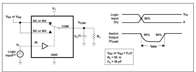
Figure 6.Break-Before-Make Time (tBBM)
