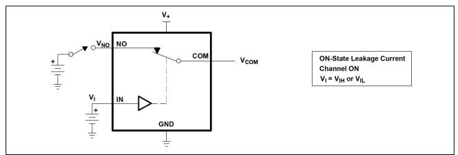
Figure 3. ON-State Leakage Current (ICOM(ON), INO(ON))
