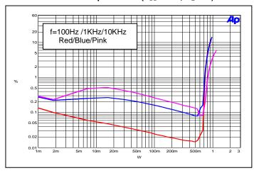
THD+N vs. Frequency ( $V_{DD}=5.0V$ ,  $R_L=4\Omega$ )
