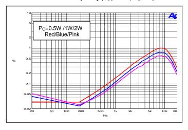
THD+N vs. Frequency ( $V_{DD}=5.0V$ ,  $R_L=8\Omega$ )
