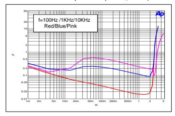
THD+N vs. Output Power ( $V_{DD}=5V$ ,  $R_L=8\Omega$ )
