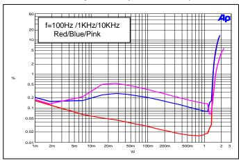
THD+N vs. Output Power ( $V_{DD}$ =3.6V,  $R_L$ =4 $\Omega$ )
