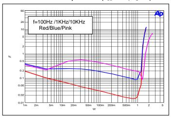
THD+N vs. Output Power ( $V_{DD}=3.6V$ ,  $R_L=8\Omega$ )
