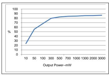
Efficiency vs. Output Power ( $V_{DD}$ =5.0V,  $R_L$ =8 $\Omega$ )
