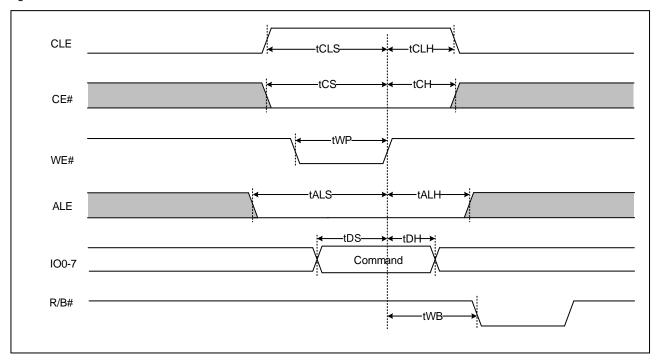
Figure 9: Command Input Cycle figures
