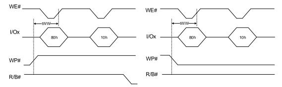
Figure 13\_a: Write Protect Disable with program figures
