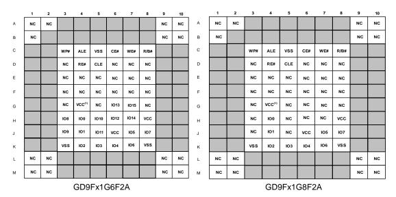
Figure 2\_a: 63-FBGA x16 device ball location figures
