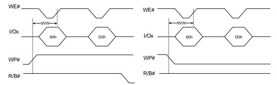
Figure 13\_c: Write Protect Disable with erase figures
