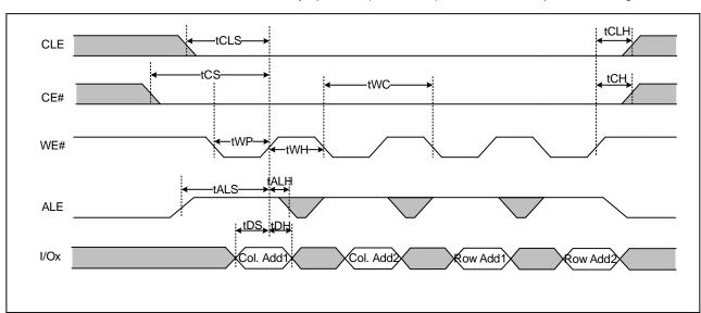
Figure 10: Address Input Cycle figures
