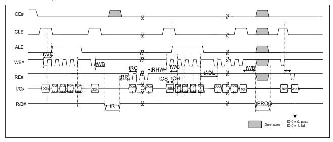
Figure 21: Copy-Back Program with Random Data Input figures
