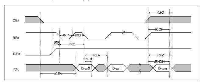
Figure 12\_b: Data Output Cycle figures
