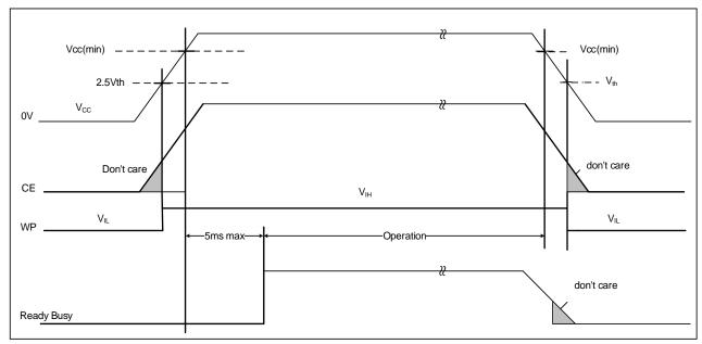
Figure 30\_a: Data protection and Power on/off (3.3V Device)
