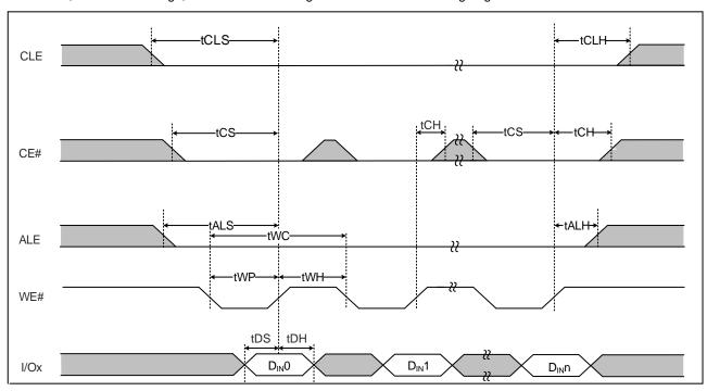
Figure 11: Data Input Cycle figures
