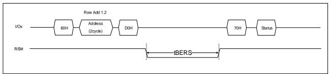
Figure 22: Common Block Erase Operation figures
