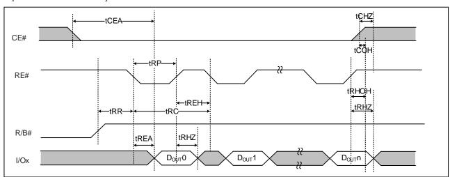
Figure 12\_a: Data Output Cycle figures
