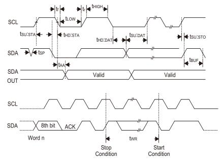
Note: The write cycle time  $t_{WR}$  is the time from a valid stop condition of a write sequence to the end of the valid start condition of sequential command.
