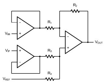
Figure 6. Instrument Amplifier
