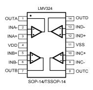
Figure 1. Pin Assignment Diagram
