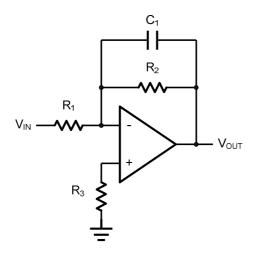
Figure 5. Low Pass Active Filter
