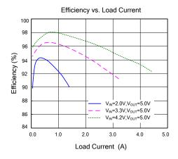
Figure 2. Efficiency Figure
