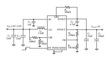
Figure 1. Schematic Diagram
