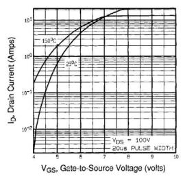
Fig. 3 - Typical Transfer Characteristics
