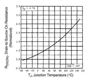
Fig. 4 - Normalized On-Resistance vs. Temperature
