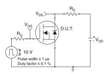
Fig. 10a - Switching Time Test Circuit
