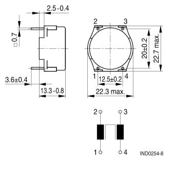
Tolerances to ISO 2768-cl / ISO 8015. Size ISO 14405 (E) All dimensions in mm
