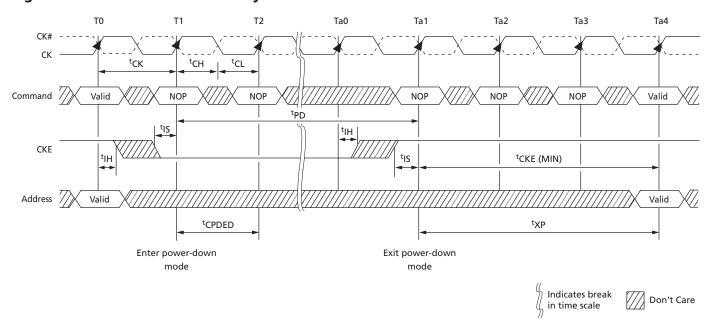
Figure 95: Precharge Power-Down (Fast-Exit Mode) Entry and Exit
