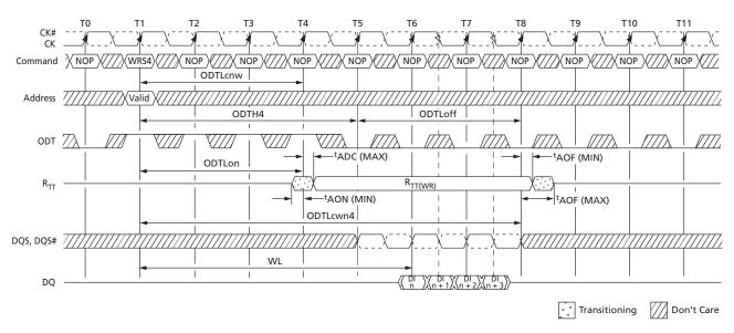
otes: 1. Via MRS or OTF. AL = 0, CWL = 5.  $R_{TT,nom}$  can be either enabled or disabled. If disabled, ODT can remain HIGH.  $R_{TT(WR)}$  is enabled.
