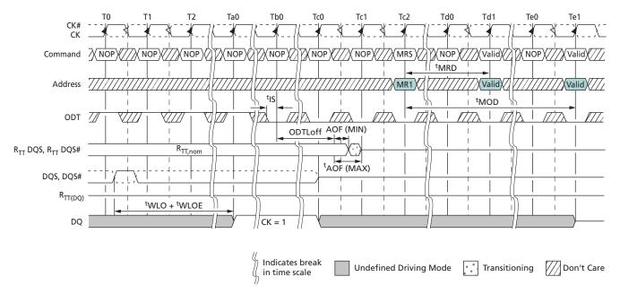
Note: 1. The DQ result, = 1, between Ta0 and Tc0, is a result of the DQS, DQS# signals capturing CK HIGH just after the T0 state.
