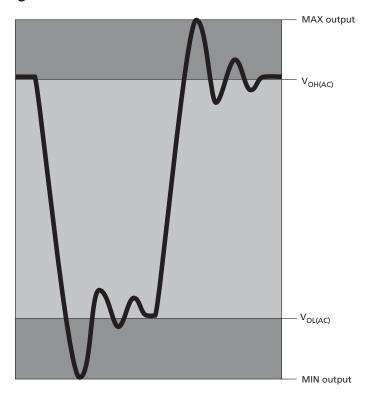
**Table 67: DDR3L Differential Output Driver Characteristics**
