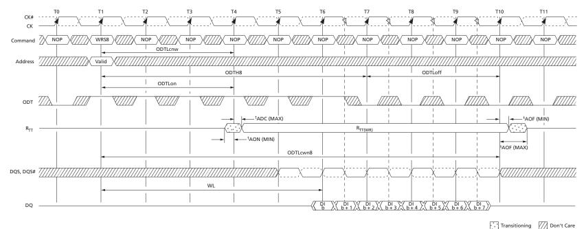
Notes: 1. Via MRS or OTF; AL = 0, CWL = 5. If  $R_{TT,nom}$  can be either enabled or disabled, ODT can be HIGH.  $R_{TT(WR)}$  is enabled.
