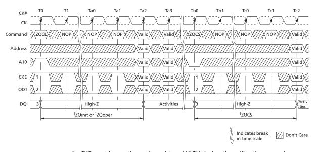
Notes: 1. CKE must be continuously registered HIGH during the calibration procedure.
