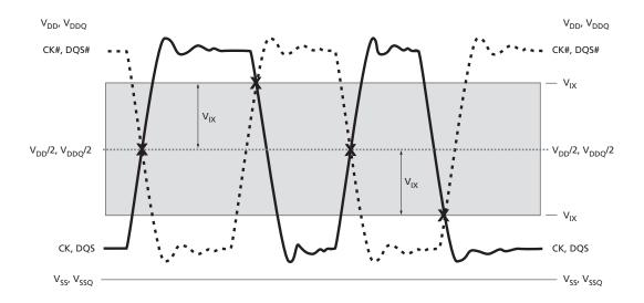
**Figure 15: Single-Ended Requirements for Differential Signals**
