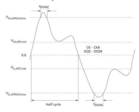
Table 47: DDR3L 1.35V - Minimum Required Time <sup>t</sup>DVAC for CK/CK#, DQS/DQS# Differential for AC Ringback
