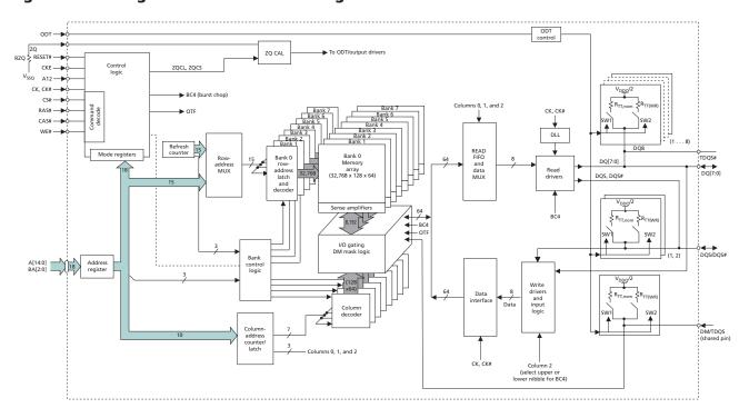
Figure 5: 128 Meg x 16 Functional Block Diagram
