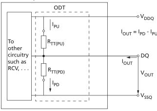
**Table 50: On-Die Termination DC Electrical Characteristics**
