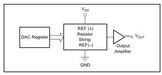
FIGURE 1. HT5320A Architecture.
