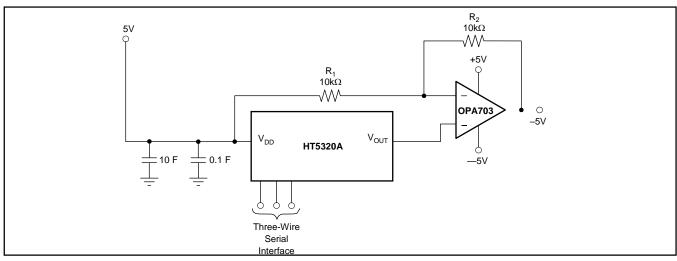
FIGURE 10. Bipolar Operation with the HT5320A.
