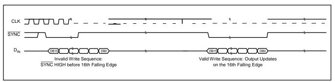
FIGURE 4. SYNC Interrupt Facility.
