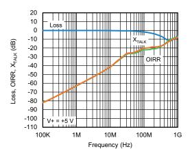
Insertion Loss, Off-Isolation Crosstalk vs. Frequency
