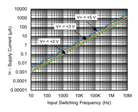
**Supply Current vs. Input Switching Frequency**
