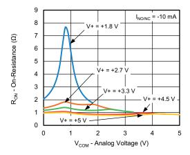
R<sub>ON</sub> vs. V<sub>COM</sub> and Supply Voltage
