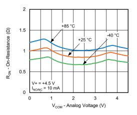
$R_{\text{ON}}$  vs.  $V_{\text{COM}}$  and Temperature
