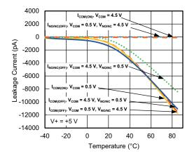
Leakage Current vs. Temperature
