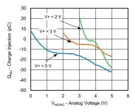
Charge Injection vs. Analog Voltage
