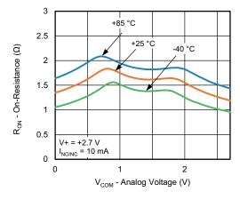
$R_{\text{ON}}$  vs.  $V_{\text{COM}}$  and Temperature
