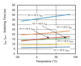
Switching Time vs. Temperature and Supply Voltage
