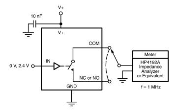
Fig. 5 - Channel Off / On Capacitance
