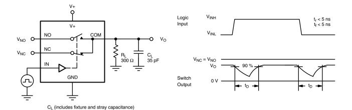
Fig. 2 - Break-Before-Make Interval
