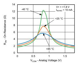
$R_{\text{ON}}$  vs.  $V_{\text{COM}}$  and Temperature
