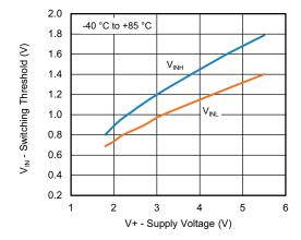
Switching Threshold vs. Supply Voltage
