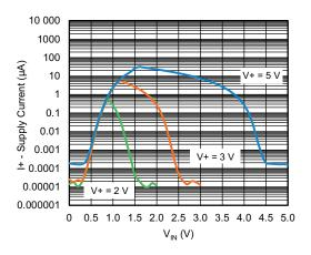
Supply Current vs. Enable Input Voltage
