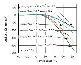
Leakage Current vs. Temperature
