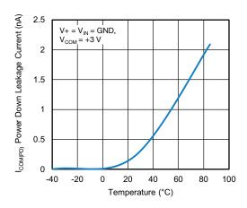
Power Down Leakage Current vs. Temperature
