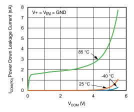
Power Down Leakage Current vs. V<sub>COM</sub>
