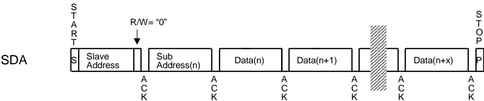
Figure 66. Data Transfer Sequence at I 2 C Bus Mode
