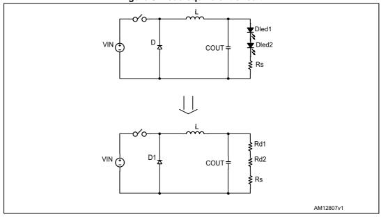
Figure 8. Load equivalent circuit
