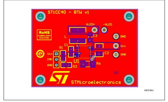
It is strongly recommended that the input capacitors are to be put as close as possible to the relative pins, see C1 and C2.
