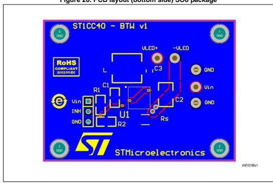
Figure 20. PCB layout (bottom side) SO8 package
