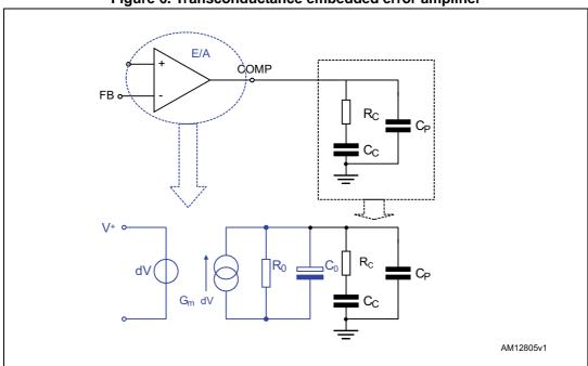
Figure 6. Transconductance embedded error amplifier
