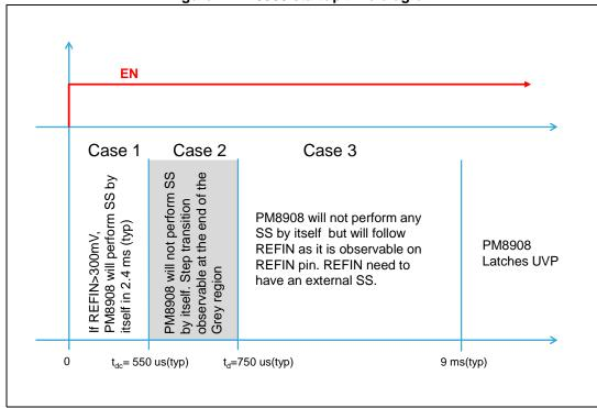
Figure 7. PM8908 startup time diagram
