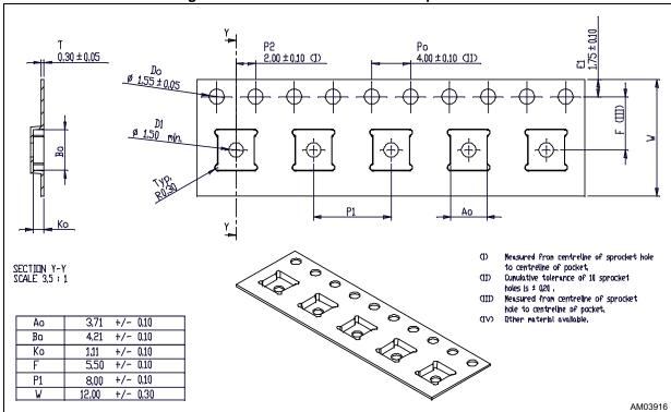
Figure 13. QFN20 3.5 x 4 x 1.0 mm tape and reel
