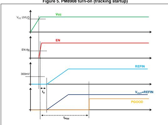
Figure 5. PM8908 turn-on (tracking startup)
