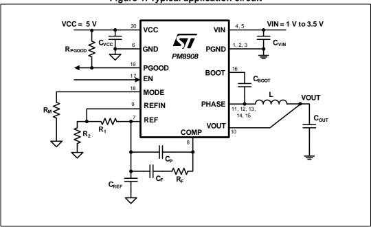
Figure 2. Typical memory termination application circuit
