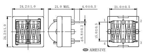
\* Dimension does not include solder used on coil.
