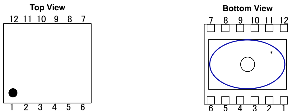
RP605K [DFN(PLP)2730-12] Pin Configuration
