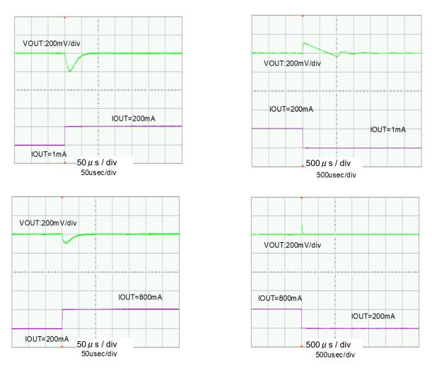
VIN=5.0V, VOUT=3.3V, MODE/SYNC=0V (PWM/PFM automatic switching control) L=4.7  $\mu$  H (CDRH4D28C), CIN=10  $\mu$  F (ceramic), CL=10  $\mu$  F (ceramic), Topr=25°C
