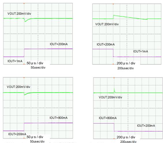
VIN=5.0V, VOUT=1.5., ... C=0V (PWM/PFM automatic switching contr  $^{21}$  L=4.7  $\mu$  H (CDRH4D28C), CIN=10  $\mu$  F (ceramic), CL=10  $\mu$  F (ceramic), Topr=25°C
