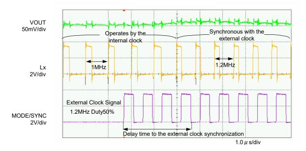
\* When an input of MODE/SYNC is changed from "L" voltage into a clock signal of 1.2MHz and 50% duty.
