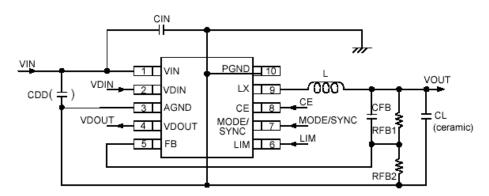
$^{(1)}A$  capacitor of 2200pF~0.1µF is recommended to place at the C<sub>DD</sub> between the AGND pin and the V<sub>IN</sub> pin. Please refer to the page showing INSTRUCTION ON PATTERN LAYOUT for more detail.
