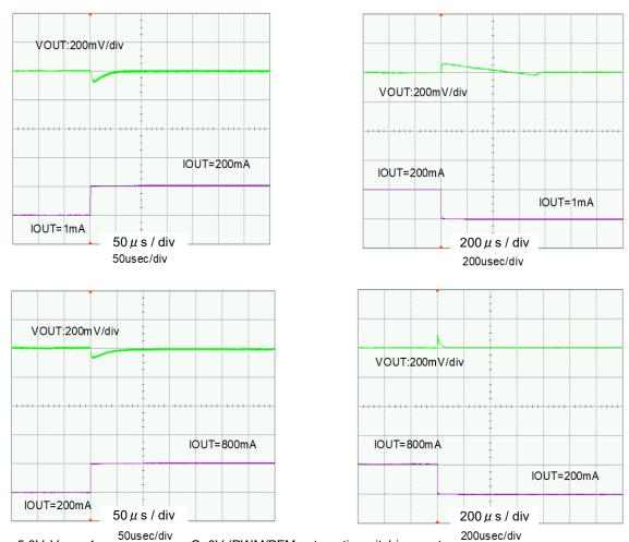
VIN=5.0V, VOUT=1. C=0V (PWM/PFM automatic switching contr L=2.2  $\mu$  H (CDRH4D28C), CIN=10  $\mu$  F (ceramic), CL=10  $\mu$  F (ceramic), Topr=25°C
