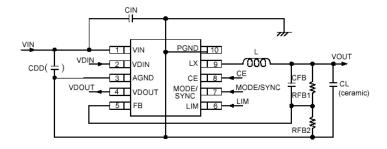
(\*1) A capacitor of 2200pF~0.1  $\mu$  F is recommended to place at the  $C_{\rm DD}$  between the AGND pin and the  $V_{\rm IN}$  pin.
