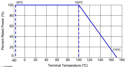
Operating temperature range of -55°C to 170°C. Storage condition:  $5^{\circ}$ C ~ 35°C, humidity of 40% ~ 75%.
