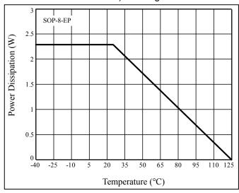
Figure 33 Dissipation Curve
