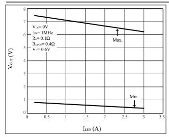
Figure 31 Minimum and Maximum Output Voltage versus LED Current (minimum  $t_{\text{ON}}$  and  $t_{\text{OFF}}$  = 150ns)
