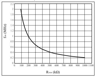
Figure 28 Operating Frequency vs. R<sub>TON</sub> Resistance
