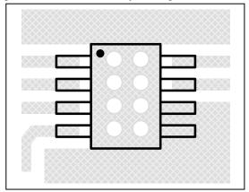
Figure 34 Board Via Layout For Thermal Dissipation
