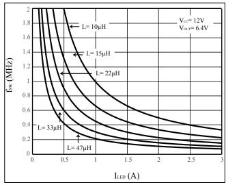
Figure 32 Inductance Selection Based On 30% Current Ripple
