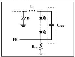
Figure 27 Adding Output Capacitor
