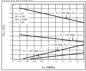
**Figure 30** Minimum and Maximum Output Voltage versus Operating Frequency (minimum t<sub>ON</sub> and t<sub>OFF</sub> = 150ns)
