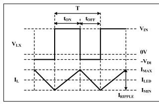
Figure 29 Operating Waveform
