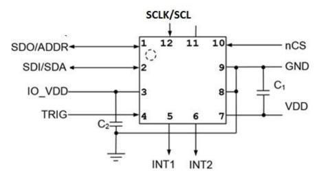
Figure 1: KX134 Application Schematic
