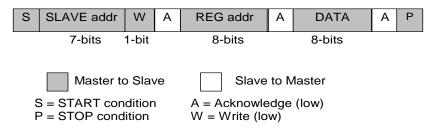
Figure 35: I<sup>2</sup>C Byte Write (SDA line)
