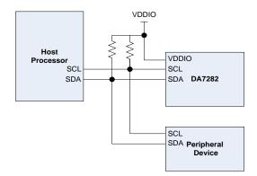
Figure 33: Schematic of the I<sup>2</sup>C Control Interface Bus
