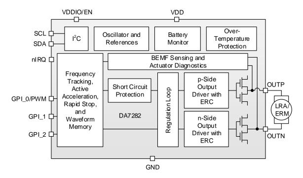
Figure 2: DA7282 Block Diagram
