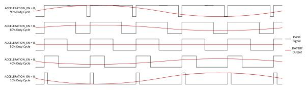
Figure 9: Example PWM Inputs with ACCELERATION\_EN = 0
