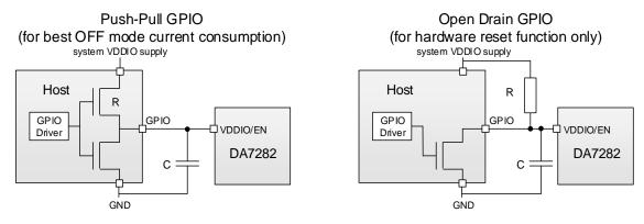
Figure 24: VDDIO/EN Pin Control in Push-Pull Configuration and Open Drain Configuration
