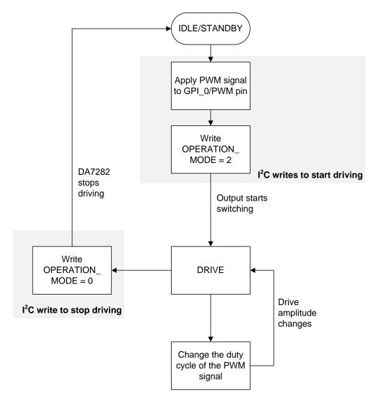
Figure 14: Operation in PWM Mode
