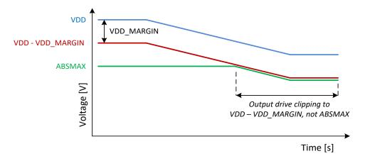
Figure 22: Automatic Output Limiting
