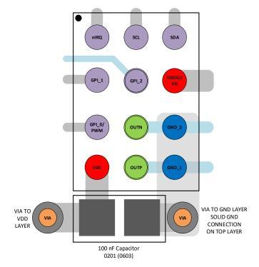
Figure 43: WLCSP Example PCB Layout
