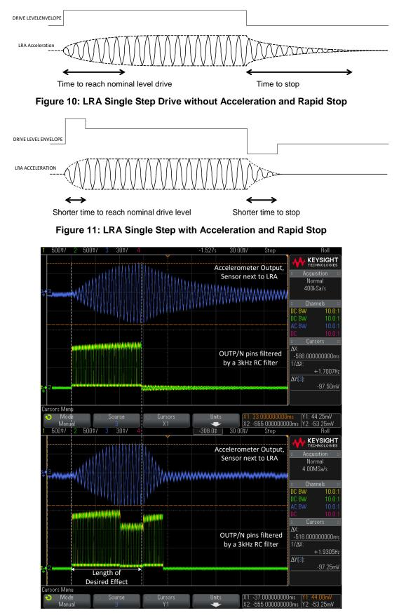
Figure 12: Simple Drive (Top) versus Active Acceleration and Rapid Stop Enabled (Bottom)DatasheetRevision 3.030-Jul-2019
