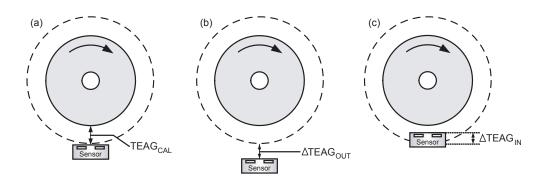
For more information on these figures and the calculations used to generate them, please refer to the Applications Note *Determining Allowable Air Gap Variation for the ATS642*.
