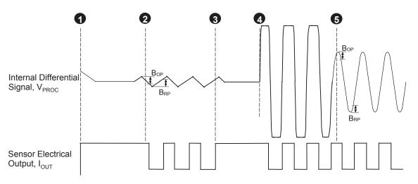
Figure 9: Operation of Running Mode Gain Adjust.
