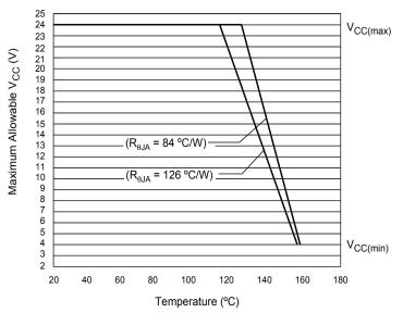
Maximum Power Dissipation, P<sub>D(max)</sub>
