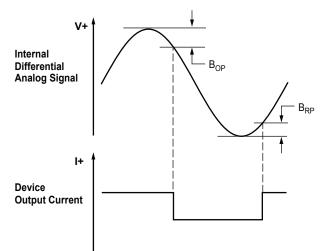
Figure 6: Peak Detecting Switchpoint Detail
