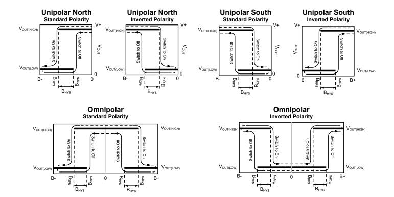
Figure 1: Hall switch magnetic and output polarity options B- indicates increasing north polarity magnetic field strength, and B+ indicates increasing south polarity magnetic field strength.
