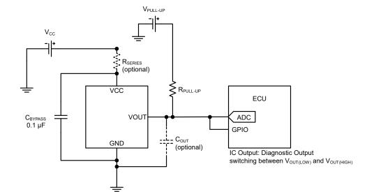
Figure 9: Typical Applications Circuits
