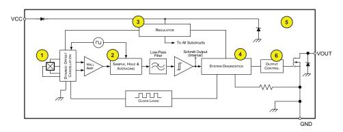
Figure 3: Diagnostics Coverage Block Diagram
