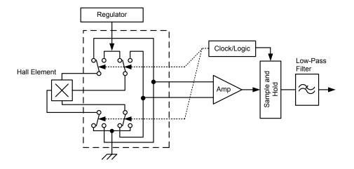
Figure 10: Model of Chopper Stabilization Circuit (Dynamic Offset Cancellation)
