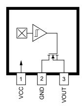
LH Package, 3-Pin SOT23W Pinout
