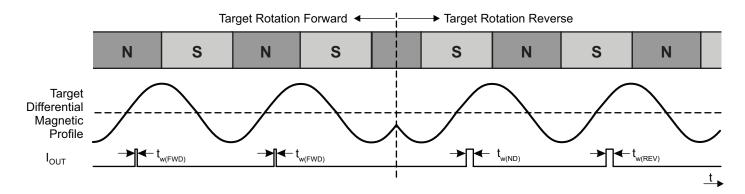
Figure 9: Example Running Mode Direction Change (-FSxxH variant)
