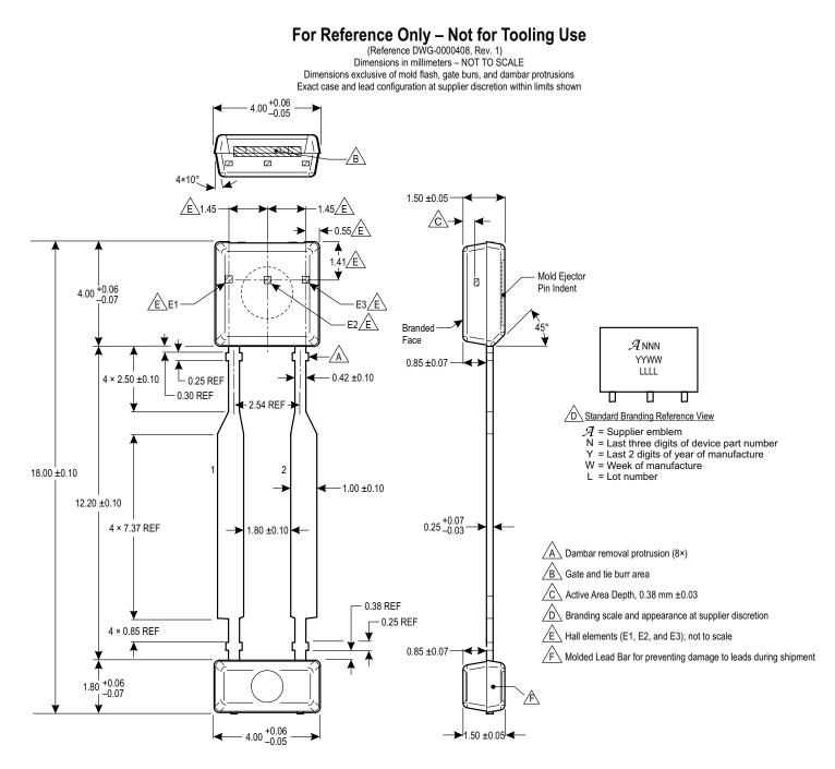
Figure 14: Package UB, 2-Pin SIP
