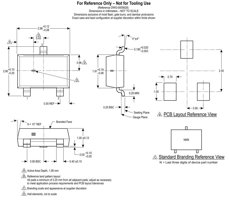
Figure 6: Package LH, 3-Pin SOT23-W
