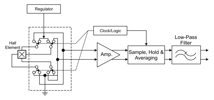
Figure 5: Model of Chopper Stabilization Circuit (Dynamic Offset Cancellation)
