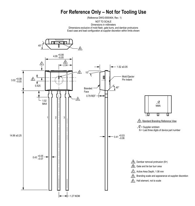
Figure 7: Package UA, 3-Pin SIP, Matrix Style
