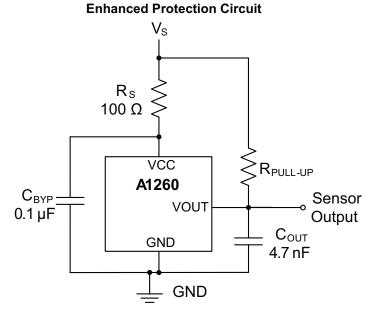
Figure 4: Typical and Enhanced Protection Application Circuits
