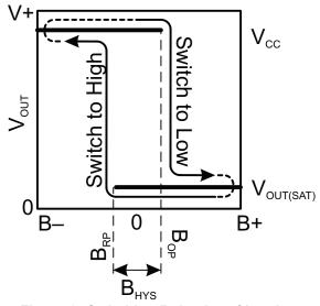
Figure 3: Switching Behavior of Latches
