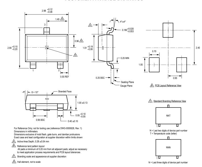
Figure 3: Package LH, 3-Pin (SOT-23W)
