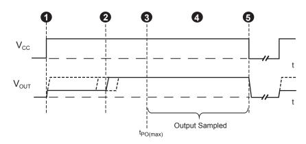
Figure 2: Continuous-Time Application,  $B < B_{RP}$
