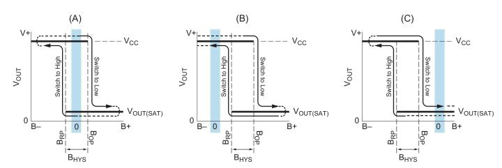
Figure 1: Bipolar Device Output Switching Modes
