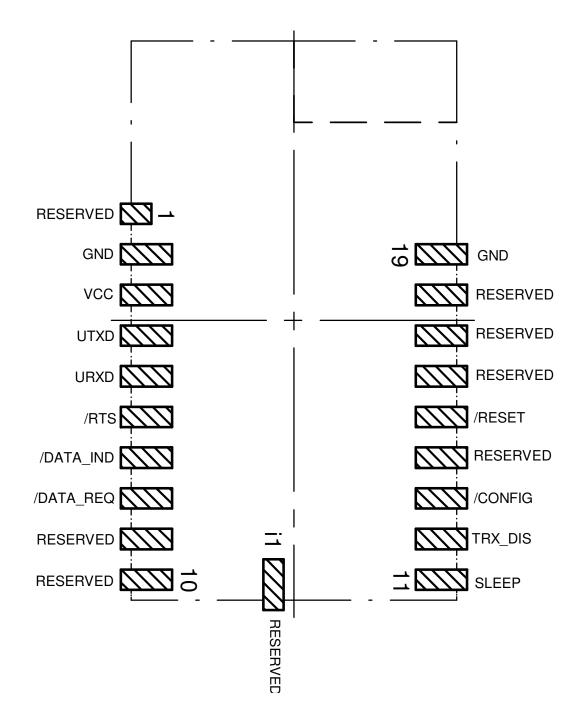
Figure 2: Pinout, internal antenna
