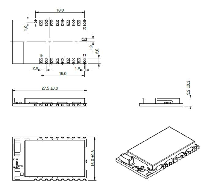
Figure 15: Module dimensions [mm]
