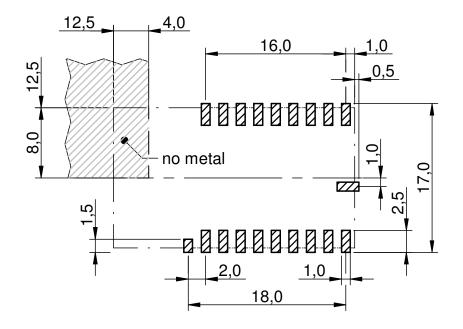
Figure 16: Footprint and dimensions [mm]
