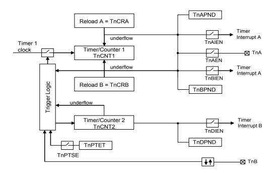
Figure 17. MFT mode 1a block diagram
