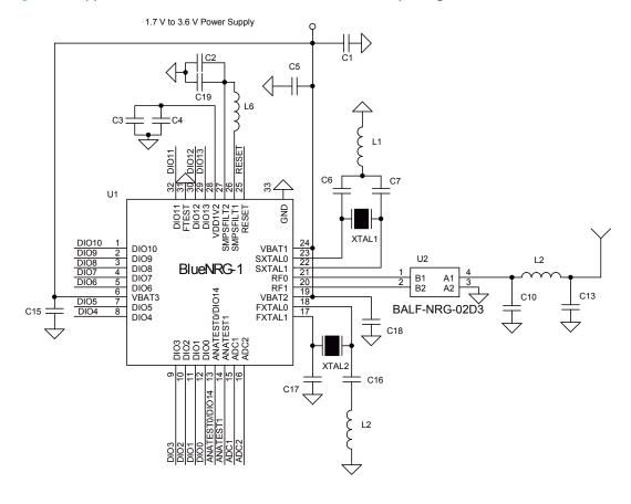
Figure 29. Application circuit: active DC-DC converter QFN32 package with BALF-NRG-02D3 balun
