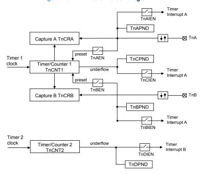
Figure 18. MFT mode 2 block diagram
