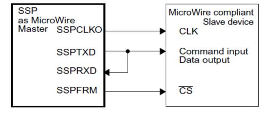
Figure 12. MicroWire master and slave communication
