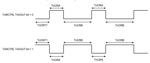
When started, the first time the Timer/Counter 1 starts with preprogrammed value in the register TnCNT1 and count down at the clock rate selected by the Timer/Counter 1 clock selector (TnCKC register). When an underflow occurs, the TnCNT1 register is reloaded alternatively with TnCRA and TnCRB registers (in this order) and counting proceeds downward from the loaded value.
