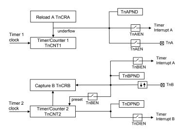
Figure 20. MFT mode 4 block diagram
