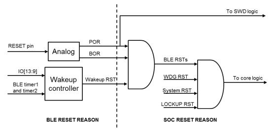
Figure 7. Reset and wake-up generation
