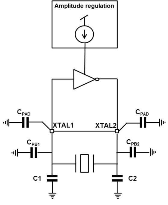
Figure 30. High speed oscillator block diagram
