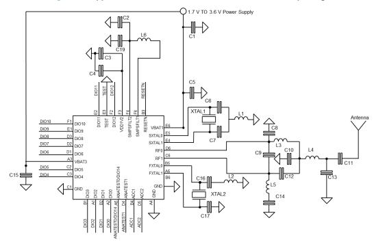
Figure 27. Application circuit: active DC-DC converter WCSP34 package
