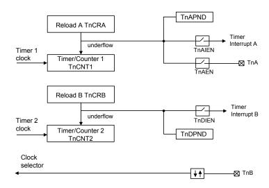
In mode 3, the Timer/Counter is configured to operate as a dual independent system timer or dual external-event counter. In addition, the Timer/Counter 1 can generate a 50% duty cycle PWM signal on the TnA pin. The TnB pin can be used as an external-event input or pulse-accumulate input, and serve as the clock source to either Timer/Counter 1 or Timer/Counter 2. Both counters can also be operated from the prescaled system clock.
