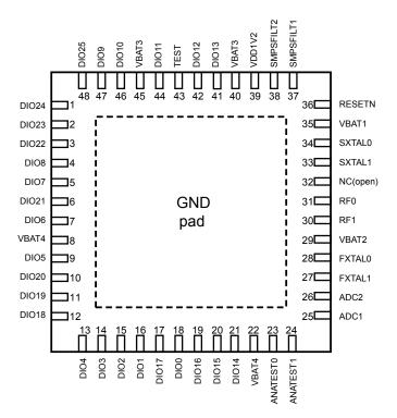
Figure 22. BlueNRG-2 pin out top view (QFN48)
