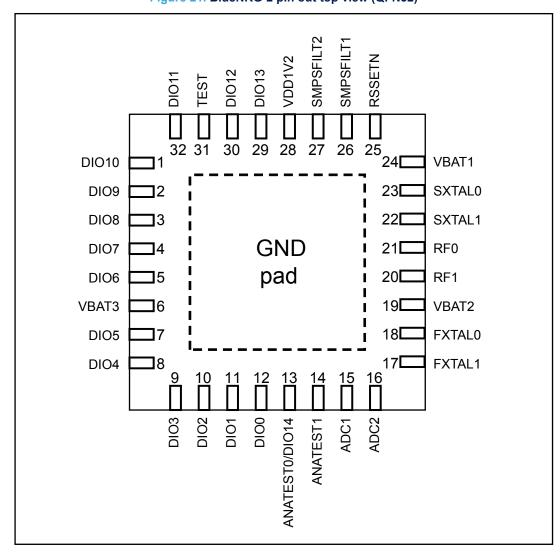
Figure 21. BlueNRG-2 pin out top view (QFN32)
