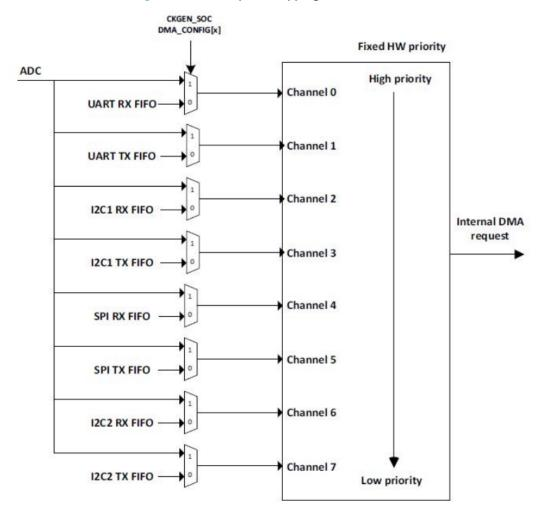
Figure 11. DMA request mapping in BlueNRG-2
