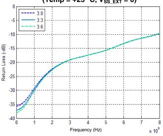
Figure 18. RFC Port Return Loss vs  $V_{DD}$ (Temp = +25 °C,  $V_{SS EXT} = 0$ )
