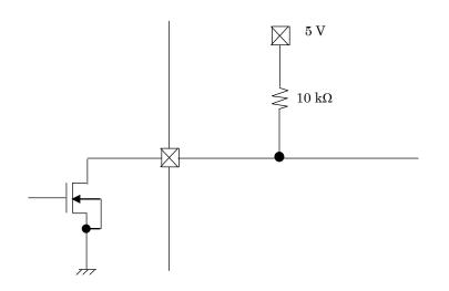
The ALERT is an open drain output pin. When the output pin is pulled up to the VCC with resistance, the low level is output (MOSFET ON) at the Reset, and the high level (internal Hi-Z) is output at the non-reset. Please connect it to the VCC.
