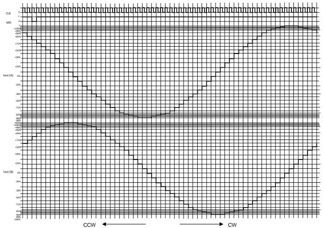
Note: MO signal is shown in the above timing chart when MO pin is connected with a pull-up resistor to VCC.
